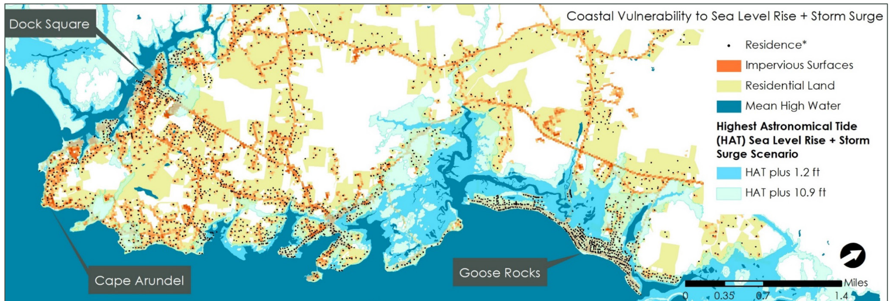
Figure 2-12 Residential land and impervious surfaces with low and high sea level rise scenarios. *The dots representing residences are derived from E-911 addresses and do not necessarily show the exact location of homes (Data Source: Maine Geological Survey, NOAA CCAP, Assessing Department)
