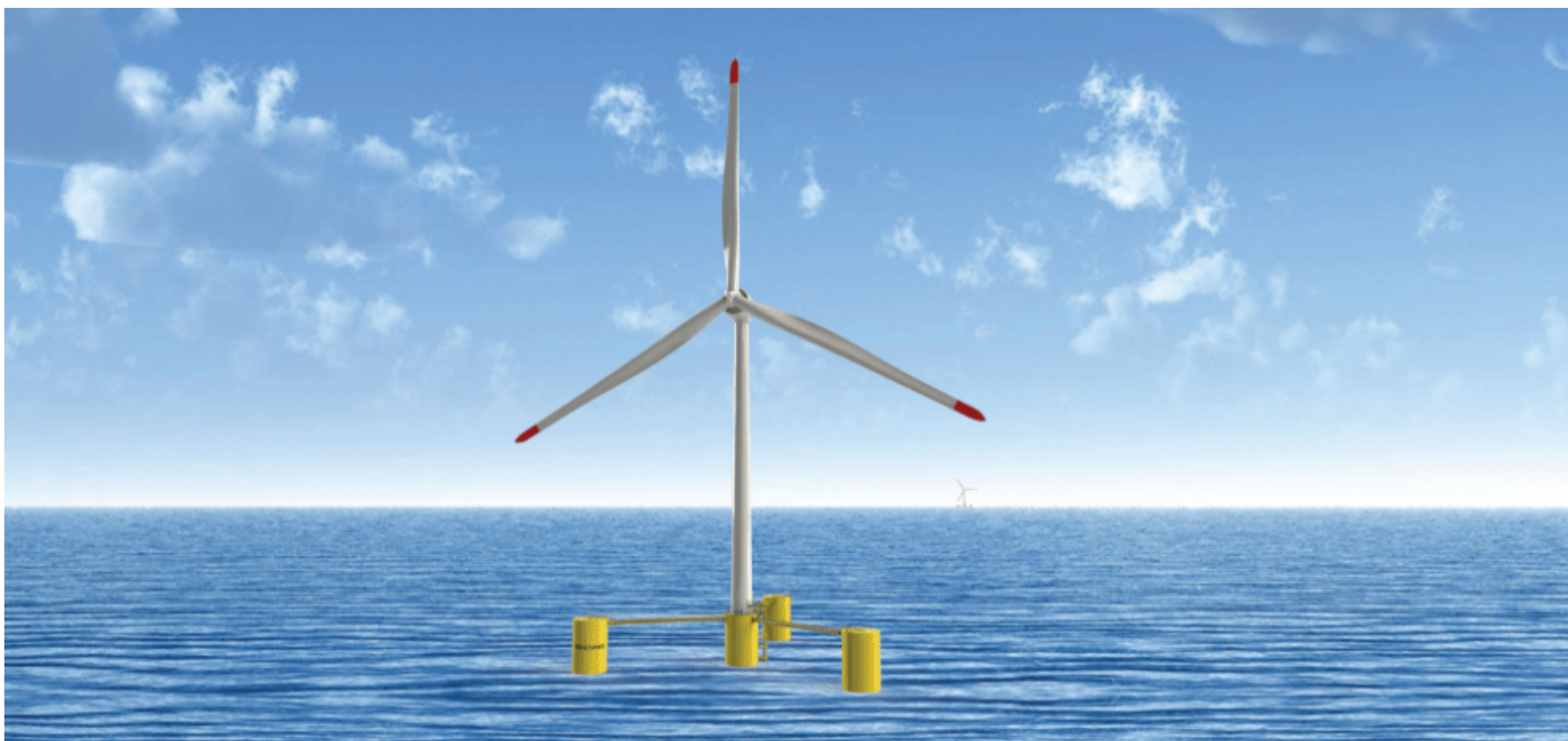
Rendering of New England Aqua Ventus, a 12 MW pilot project 3 miles off of Monhegan Island. Courtesy of the University of Maine's Advanced Structures Composites Center.
