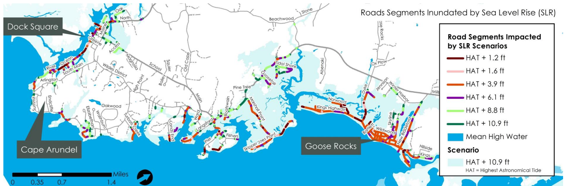
Figure 11-18. Road segments inundated by Sea Level Rise (SLR) under six SLR scenarios. The color displayed represents the highest scenario that the road is vulnerable under. A segment that is vulnerable under a 6.1 ft scenario is also vulnerable under the lower scenarios of the 1.2 ft, 1.6 ft, and 3.9 ft scenarios, for example.
