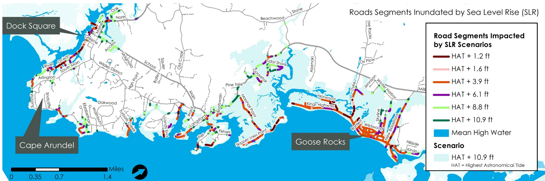
Figure 18-15. Road segments inundated by Sea Level Rise (SLR) under six SLR scenarios. The color displayed represents the highest scenario that the road is vulnerable under. A segment that is vulnerable under a 6.1 ft scenario is also vulnerable under the lower scenarios of the 1.2 ft, 1.6 ft, and 3.9 ft scenarios, for example. (Source: ME Geological Survey)
