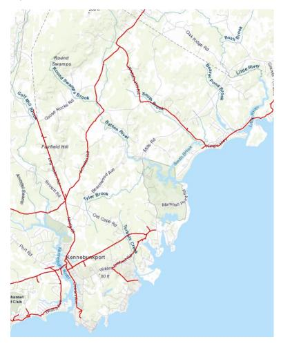
Figure 13-9 3-Phase Circuit Map, courtesy of CMP
