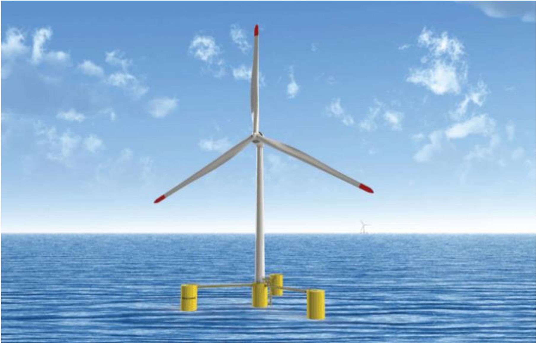
Rendering of New England Aqua Ventus, a 12 MW pilot project 3 miles off of Monhegan Island. Courtesy of the University of Maine's Advanced Structures Composites Center.
