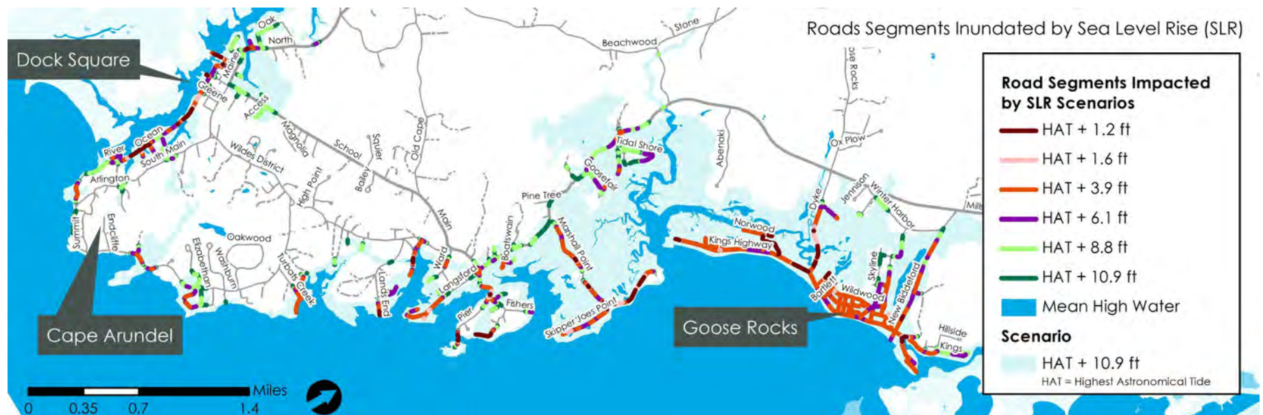
Figure 11-21. Road segments inundated by Sea Level Rise (SLR) under six SLR scenarios. The color displayed represents the highest scenario that the road is vulnerable under. A segment that is vulnerable under a 6.1 ft scenario is also vulnerable under the lower scenarios of the 1.2 ft, 1.6 ft, and 3.9 ft scenarios, for example. (Source: ME Geological Survey)
